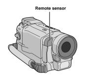
When using the remote control, be sure to point it at the remote sensor. The transmitted beam's approximate effective distance for indoor use is 5m.
